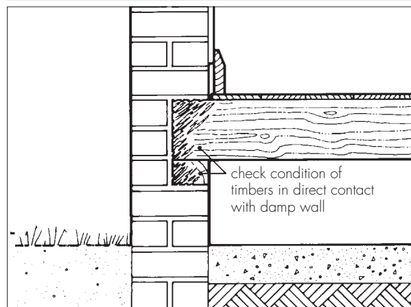
Figure 2 Check embedded timber for decay
